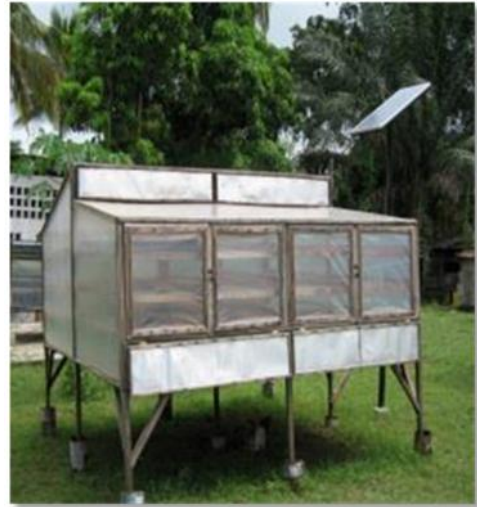
United Republic of Tanzania – Sun dryer manufactured by Claphijo Enterprises. Photo courtesy of Clara Ibihya
