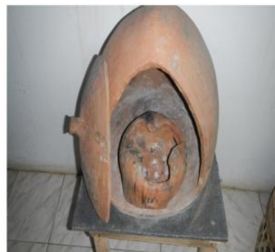
Charcoal-fired clay oven-dryer displayed at the Sharefair in Nairobi. Photo courtesy of Amal Magzoub
