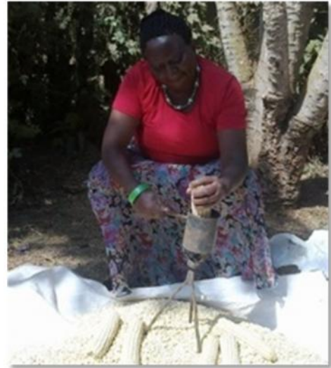
Kenya – The maize sheller is easier, faster and more hygienic than the traditional method of shelling. Photo courtesy of David Ngige
