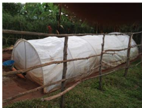
Rwanda – Flexi Biogas systems piloted in the IFAD-funded Kirehe Community-based Watershed Management Project (KWAMP). Photo courtesy of ©Antonio Rota
