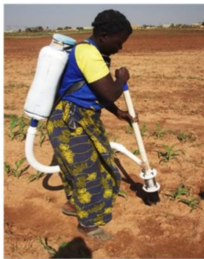
Zambia – Farmer testing the spot fertilizer applicator in her field. Photo courtesy of Musenga Silwaw
