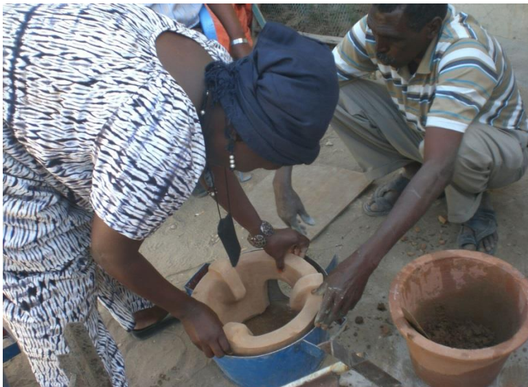
Janet of Keyo women group training a male upcoming entrepreneur on how to clad an improve cook stove
