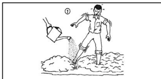
Mixing clay manually (source: A Manual for Stove-makers)
